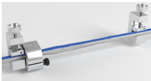
Circular cut between the spacers for a repair with 200 mm DuctRepair-Block
