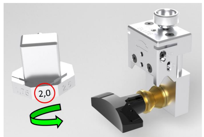
2.1.9 Twist dial of gauge for adjustment of cutting depth till the required wall thickness of microduct appears, i.e. 2.0 mm.
