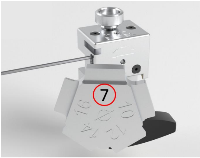
2.1.3 Remove the gauge for adjustment of outer diameter from the toolbox and insert it with the required external diameter of the microduct, i.e. 7 mm.
