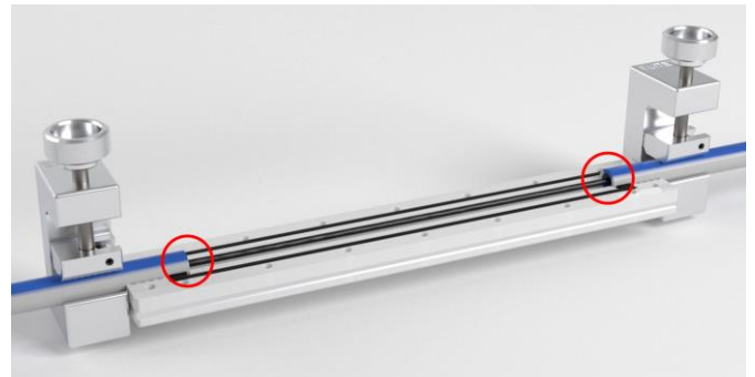
2.7.1 The ends of the microducts and the cable must be entire clean. Insert the microduct ends into the recesses in the DuctRepair-Block bottom part.
