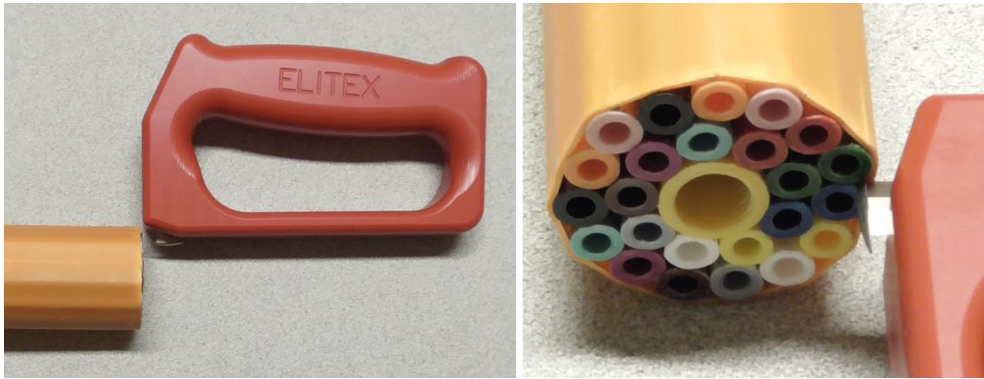
1.3 Dismantle duct bundle from jacket/sheet up to marked position. Use for this operation a tool recommended by duct manufacture. If no special tool is required, the safety jacket stripper from Elitex is recommended.
